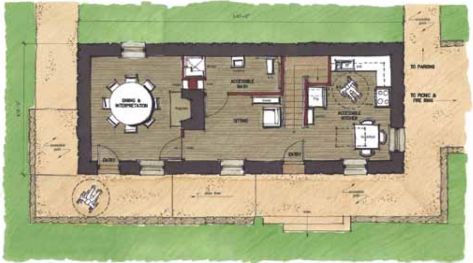
The first floor plan shows the ramp that would make the lockhouse handicap-accessible.
